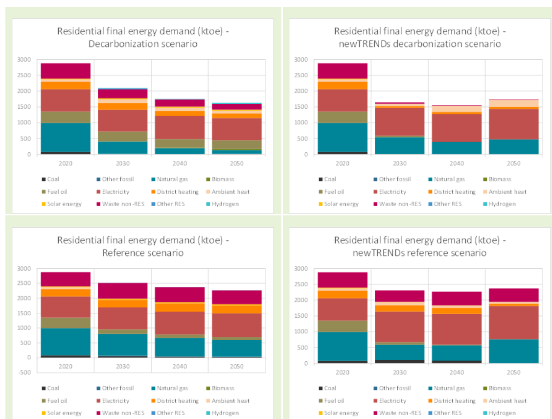
Figure 68 Prosumer model: final energy demand (ktoe) per energy carrier for the residential sector in the EU countries across scenarios
