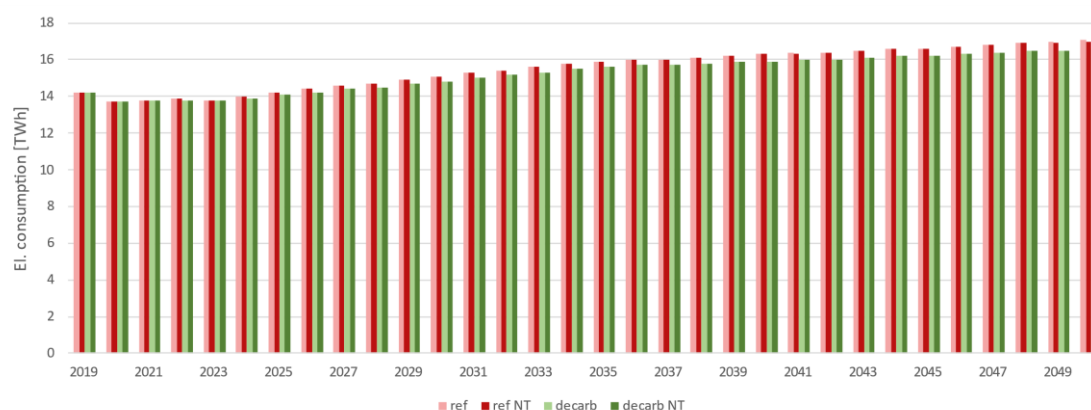
Figure 55 Electricity consumption in tertiary sector (EU27) for ICT office devices (only DC effects)
