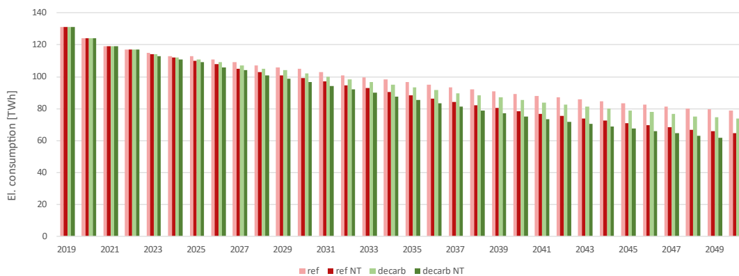
Figure 50 Final energy demand in the retail subsector (EU27) for space heating and domestic hot water applications (only EC effects)
