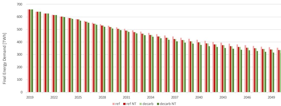
Figure 45 Final energy demand in the tertiary sector (EU27) for space heating and domestic hot water applications (only TW effects)
